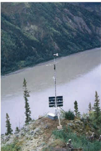
Remote tracking station used to collect and access telemetry data for radio-tagged Chinook salmon in the Yukon River basin. (Eiler, NMFS)
