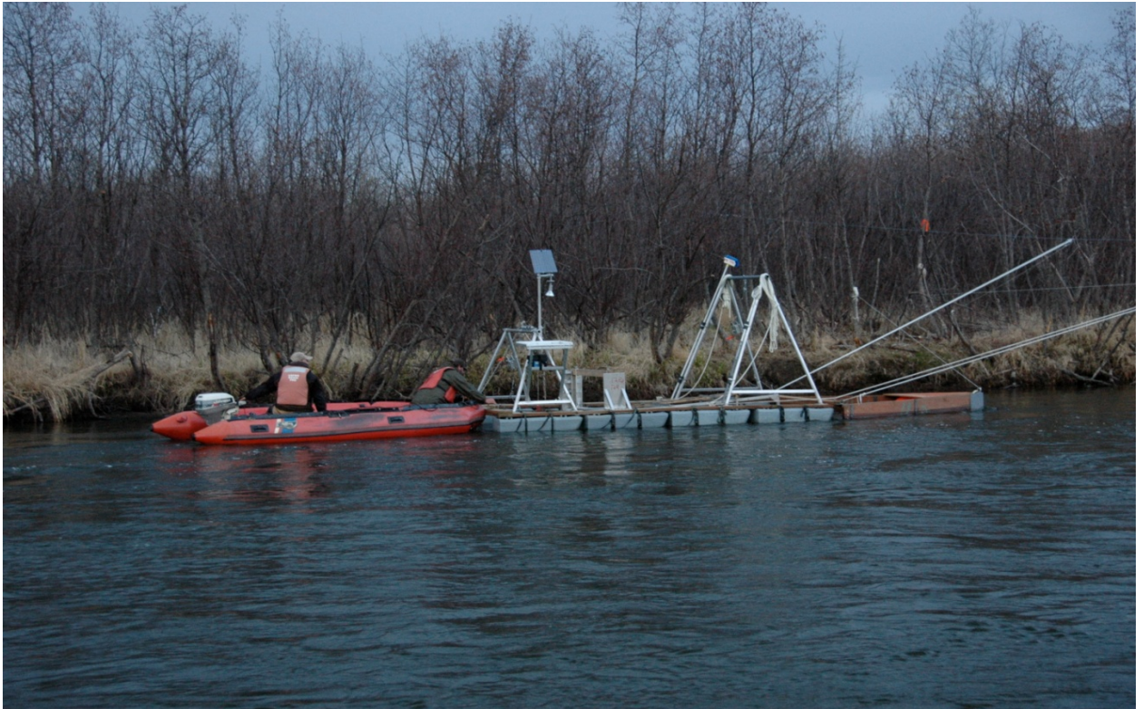
Figure 4. Inclined plane trap with ice-breaker bow attached, Kwethluk River, Alaska.
