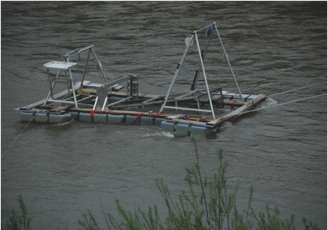
Figure 3. Photo of floating inclined plane trap as used on the Kwethluk River, Alaska.
