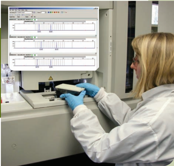
Sequencer (lower right) used to visualize coho salmon genotypes (upper left). (Crane, USFWS)
